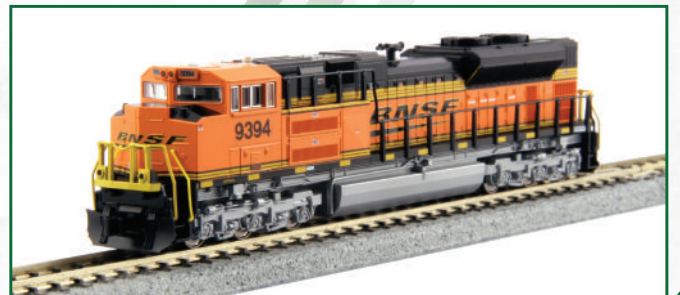
▲ The EMD SD70ACe is the latest in the long-running "70" series of engines from EMD, with a distinctive notched nose design and elevated airhorn making it immediately recognizable from above.
