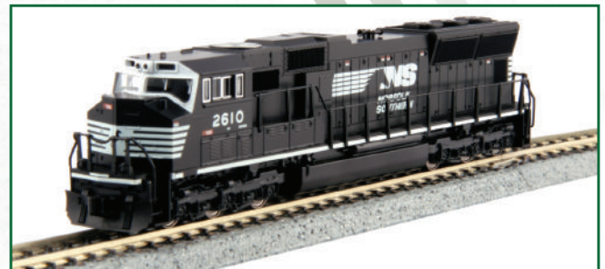
▲ The EMD SD70M is a DC powered engine, notable by the lack of inverter cabinets immediately behind the cab on the left side. Despite the lower traction, DC engines are still popular with railroads for their ease of maintenance.
